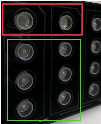
Figure 1: The top two tubes are considered defective (flat bottom). The bottom six tubes are nondefective (conical).
