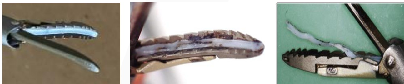
Figure 2. Example of THUNDERBEAT™ Probe in accordance with specifications (Left), Tissue Pad Deformation (Center), Tissue Pad Detachment (Right)
